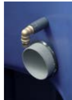
Detail of spray nozzle for starch inlet
