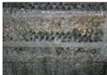
Detail of coalescing filter heavily clogged with sludge and requiring maintenance
