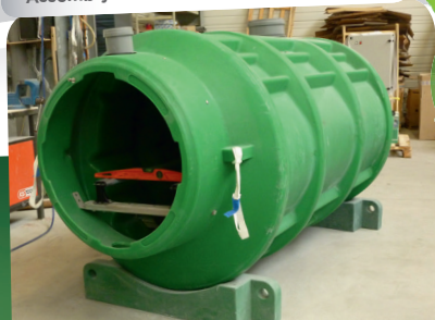
Assembly of Star 1000 pumping stations
