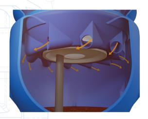
One of the many strengths of the Decant'eau is the flow distribution in the lower part of the diffuser head, which incorporates a system of guiding nozzles.
