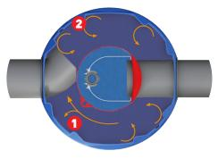
The DECANT'EAU is composed of a spreader head and a sludge tank.
