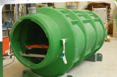
Assembly of Star 1000 pumping stations
