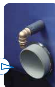
Detail of the spray nozzle for starch inlet
